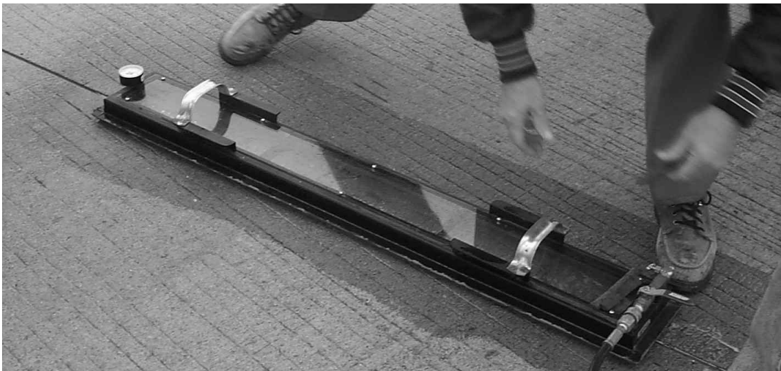
Figure 2: Seal testing on concrete test pavement using the IA-VAC device
