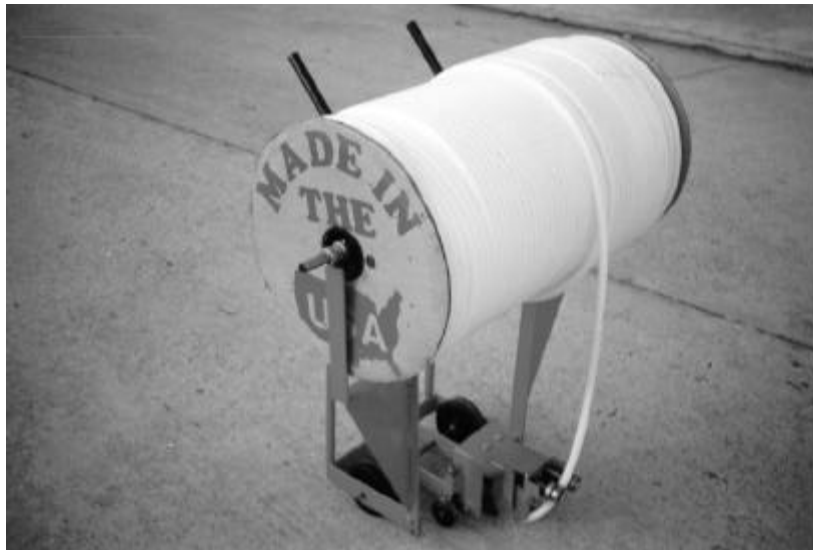
Figure 11. Automated backer rod installation tool.
