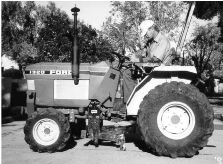
Figure 6. Undercarriage-mounted joint plow.
